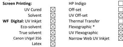
\* Flexographic Printing requires a topcoat. WVG000113 and WVF010516 have been approved by ACTEGA Coatings and Sealants (ww.altana.com) as in-line coat-able ink primers.
